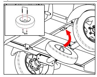
Install *Spare Tire* by first assembling the *u-bolt* though two holes in the spare. Add the *spacers* and **just** start to screw on the *angled keepers*. Then hook the *u-bolt* onto the bracket beneath the *deck* and continue to tighten the *keepers*. Once snug, insert *safety pin* in *keeper* holes. Parts:
